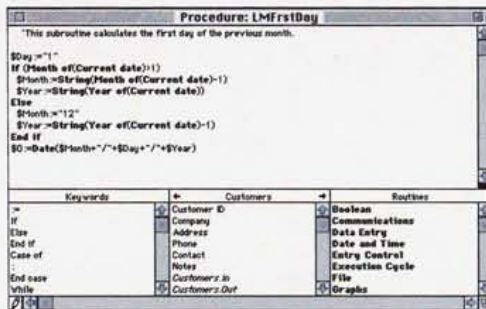
The Procedure Editor is where you write scripts and other types of procedure. The example shown here is a global procedure which defines a calculation formula.
