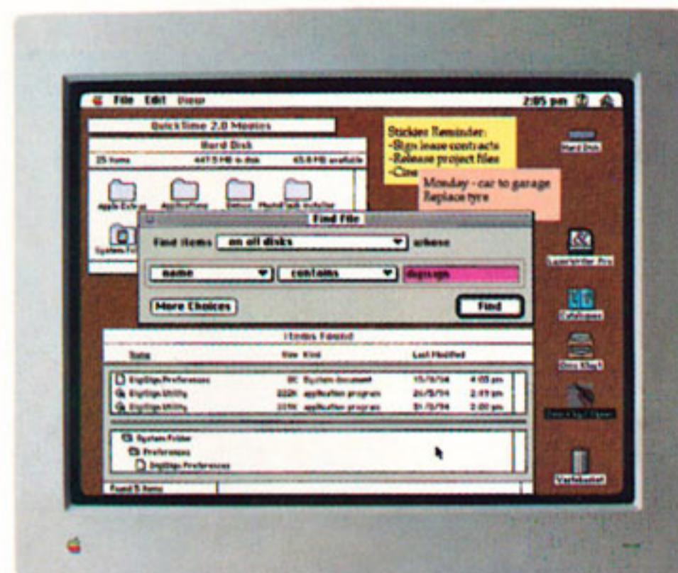
Features: Find File, Stickies and WindowShade. Desktop printer and PowerTalk icons on desktop.
