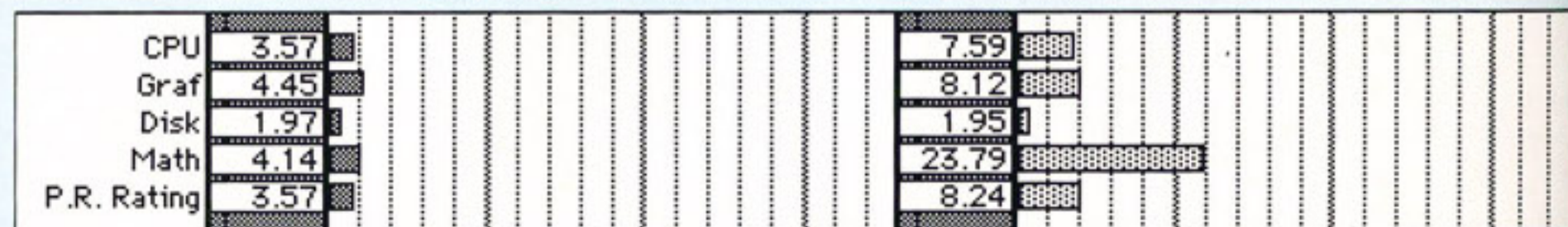
Here are the results from the Pro33 LC (right) compared to the standard LC (left).
