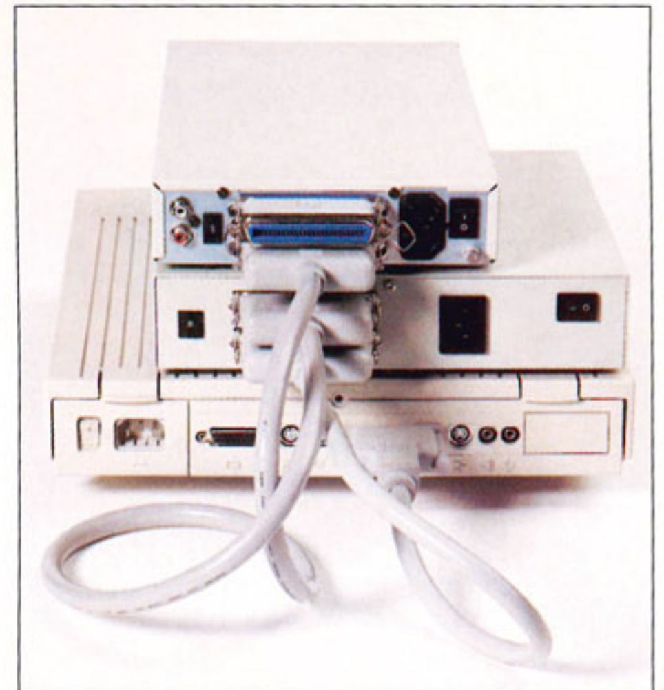
A typical SCSI daisy chain: the CD-ROM drive plugs into the SyQuest drive, which is plugged into the Mac. The terminator at the top marks the end of the chain. Note that the ID numbers of the two devices can be reset but must remain different. They don't need to be connected in numerical order.
